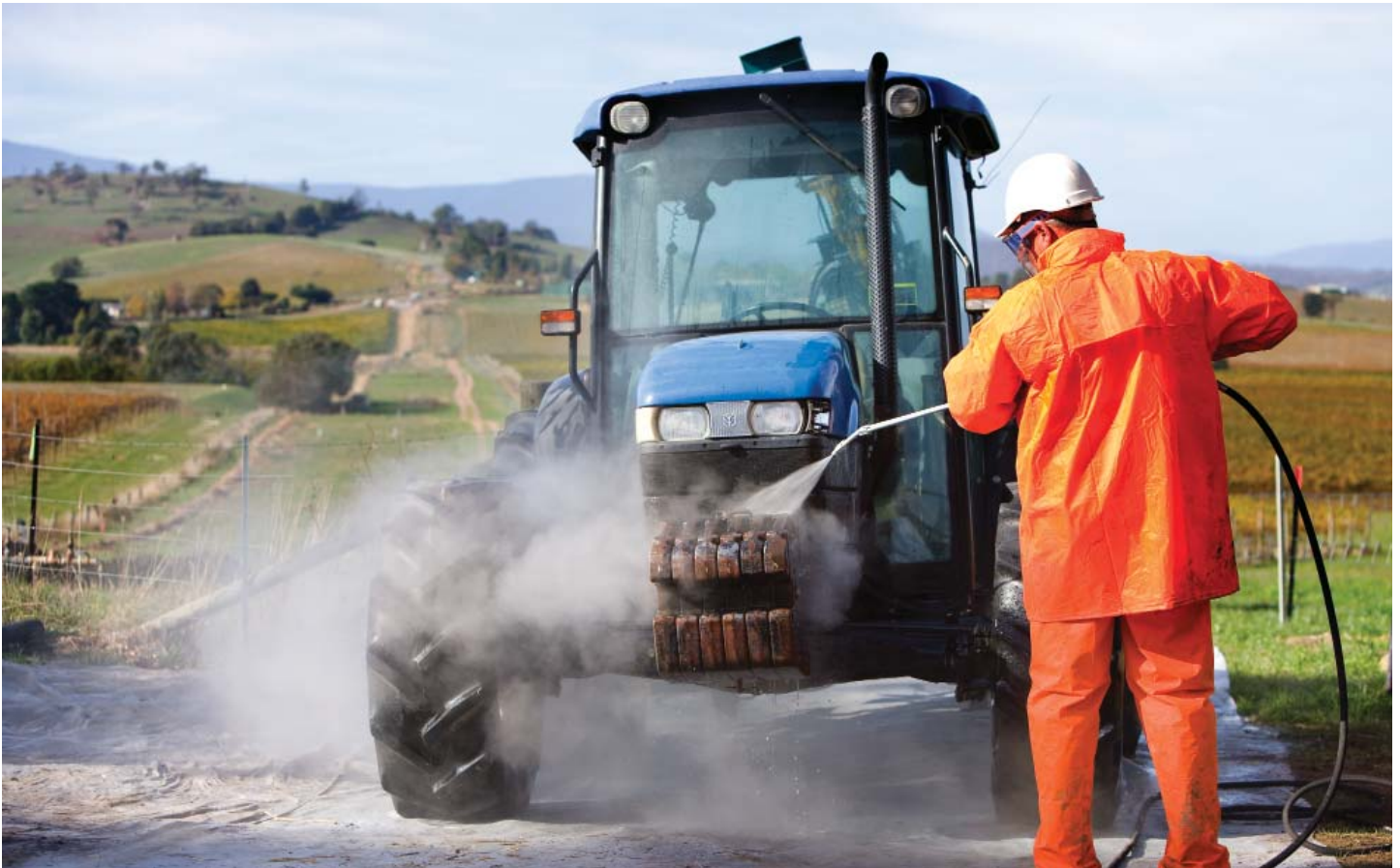
A Sugarloaf Pipeline Alliance worker steam cleans a vehicle to ensure livestock and plant diseases are not transferred between properties
